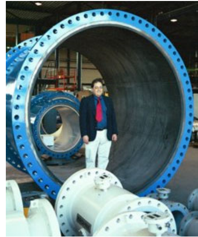
Dr. Yoder inside an 86-inch magnetic flowmeter
