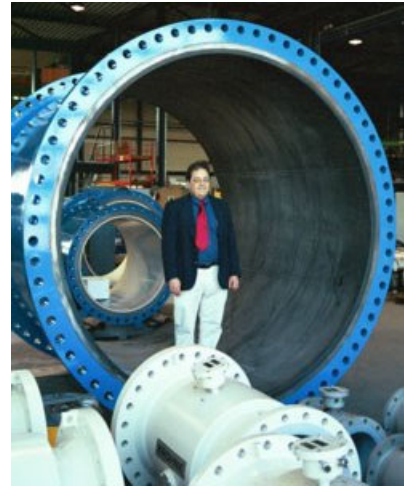
Dr. Yoder inside an 86-inch magnetic flowmeter
