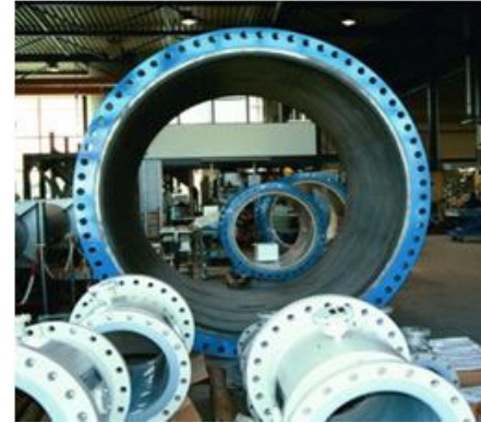
Magnetic flowmeters – Photo from the Flow Research archive.
