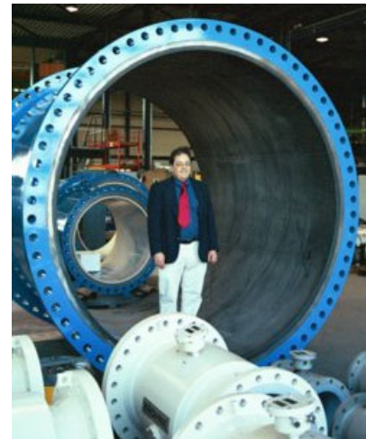
Dr. Yoder inside an 86-inch magnetic flowmeter
