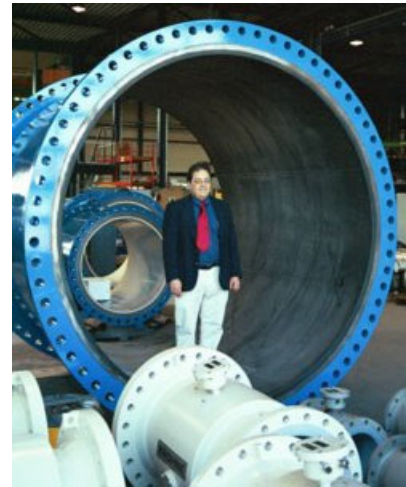
Dr. Yoder inside an 86-inch magnetic flowmeter
