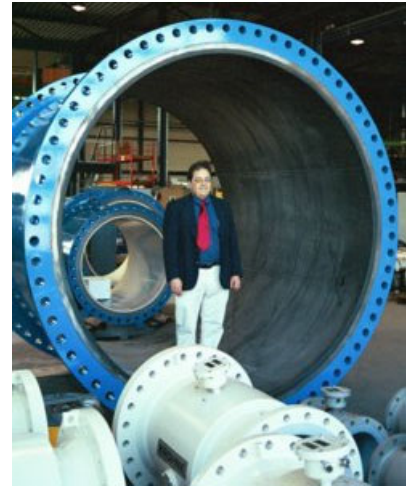
Dr. Yoder inside an 86-inch magnetic flowmeter
