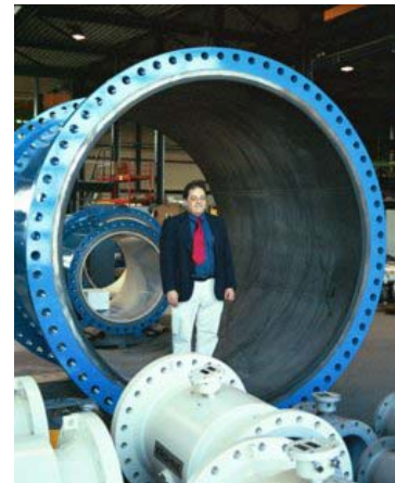
Dr. Yoder walking inside an 86 inch magnetic flowmeter
