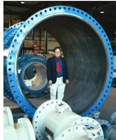
Dr. Yoder inside an 86-inch magnetic flowmeter
